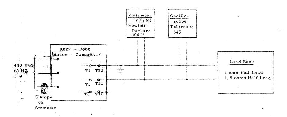
Figure 1 - Motor Generator Load Test Setup
