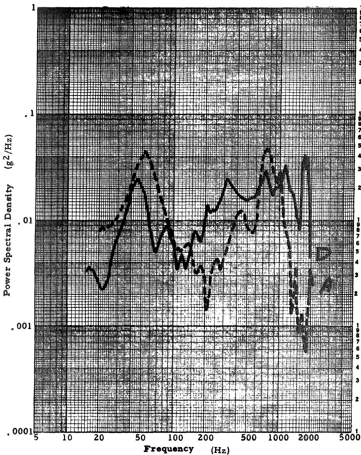
440-91 Note: Qual. SA data determined by applying a factor of 1.69 to accept level data.
