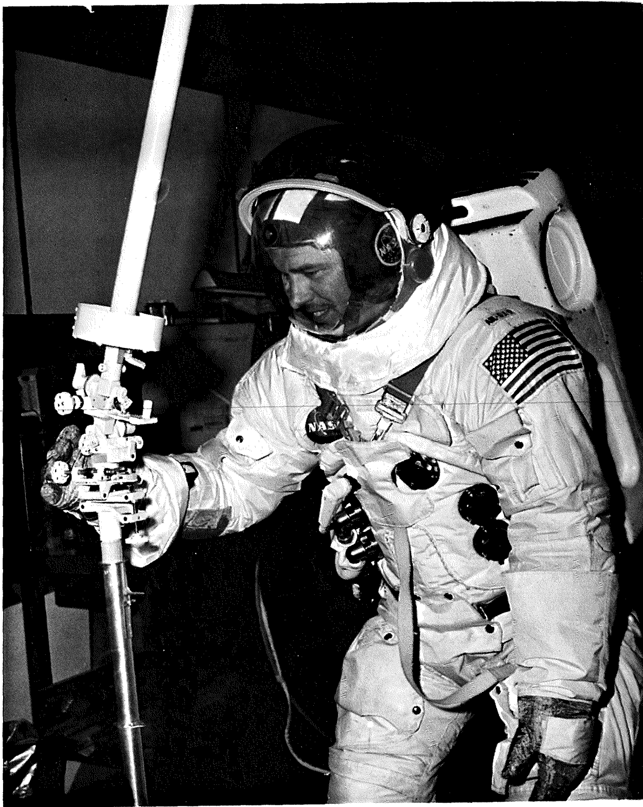
Figure 11. Antenna Aiming Mechanism Latitude Operations (Primary Mode).
