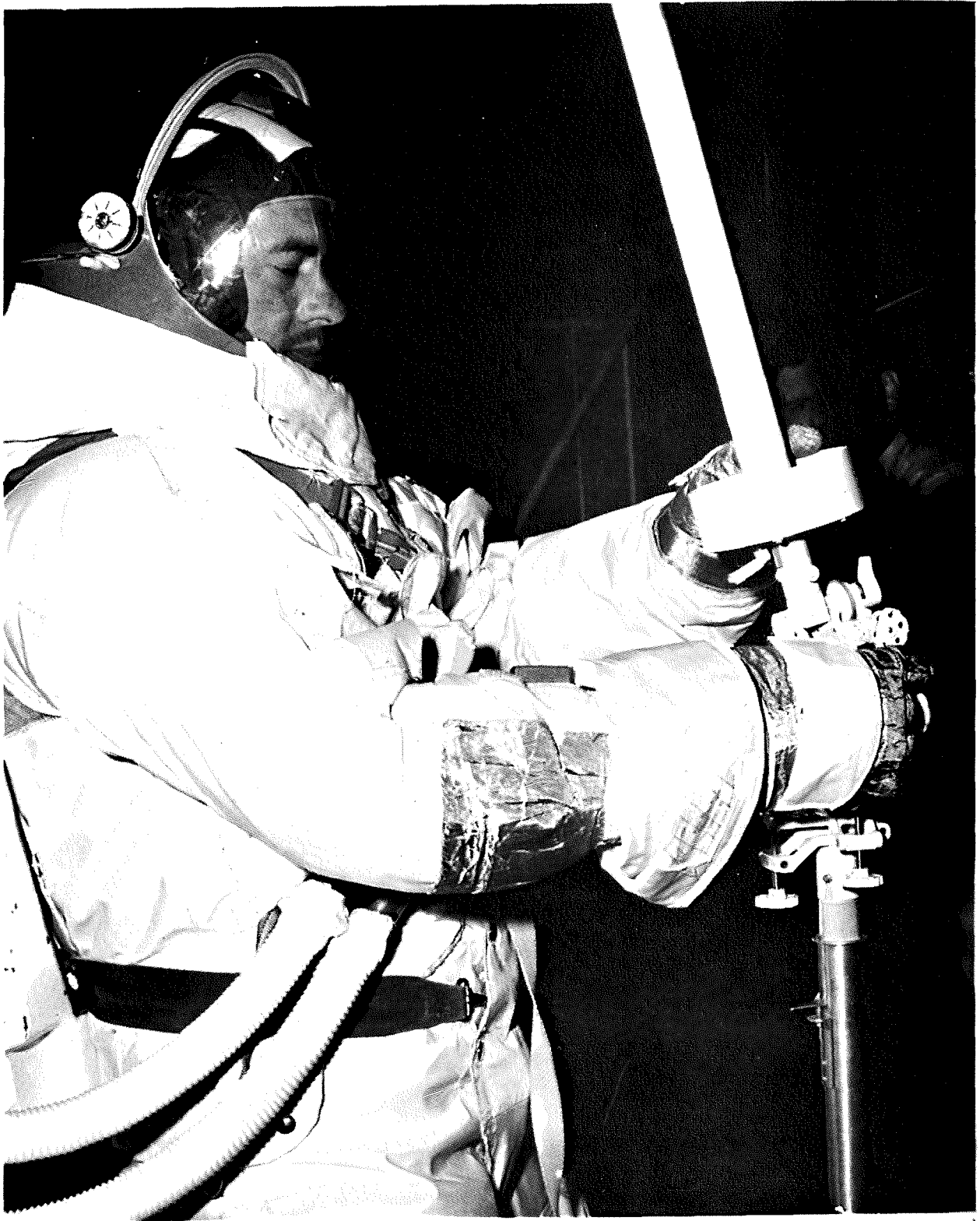
Figure 17. Antenna Aiming Mechanism Alignment Operations (Contingency Mode).
