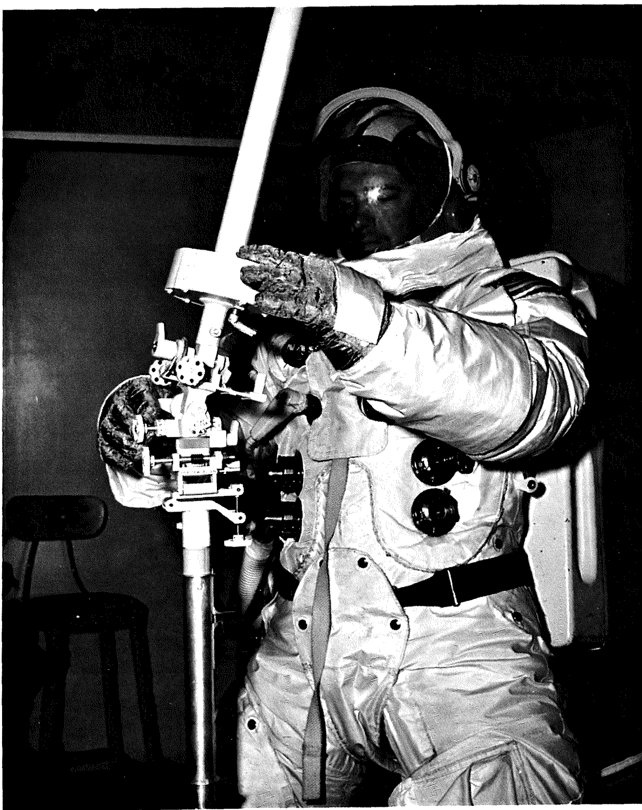
Figure 16. Antenna Aiming Mechanism Latitude Operations (Contingency Mode).
