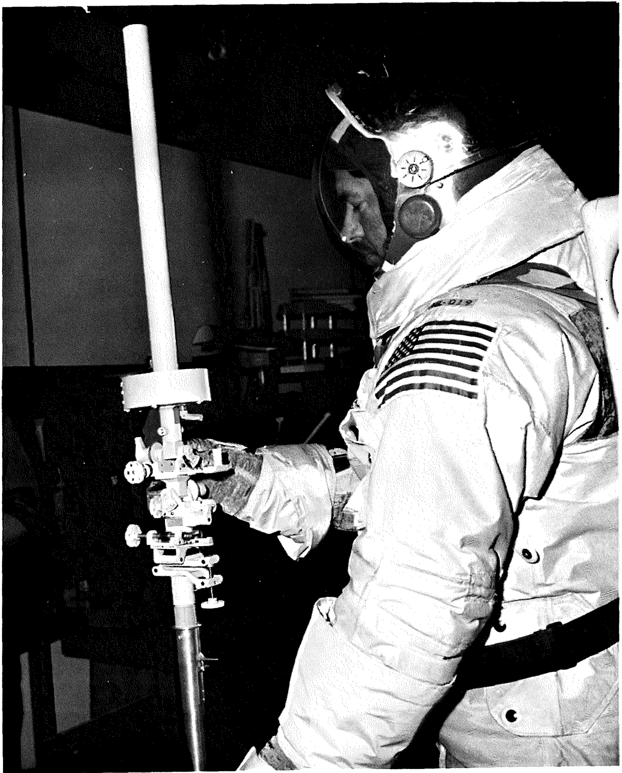
Figure 10. Antenna Aiming Mechanism Longitude Operations (Primary Mode).
