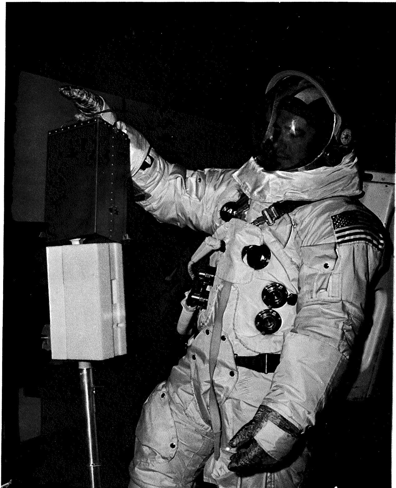
Figure 7. Antenna Aiming Mechanism Housing Removal.
