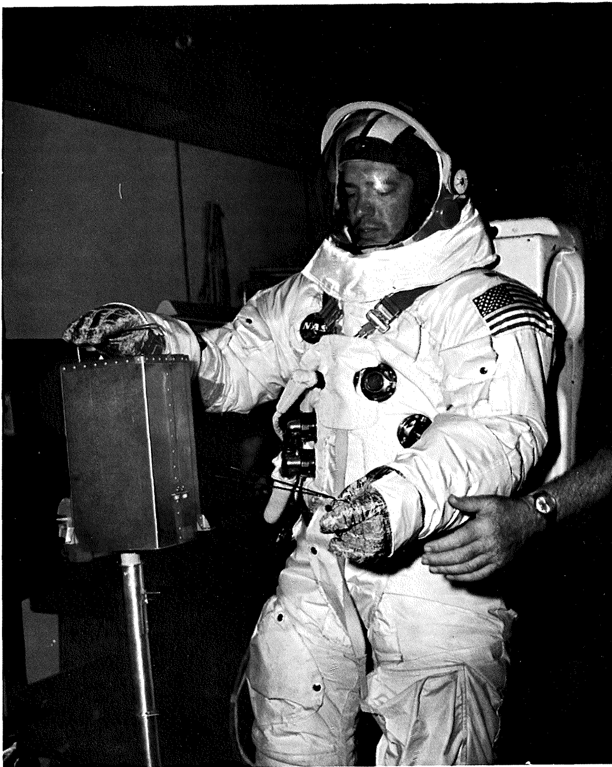
Figure 6. Antenna Aiming Mechanism Housing Pin Removal.
