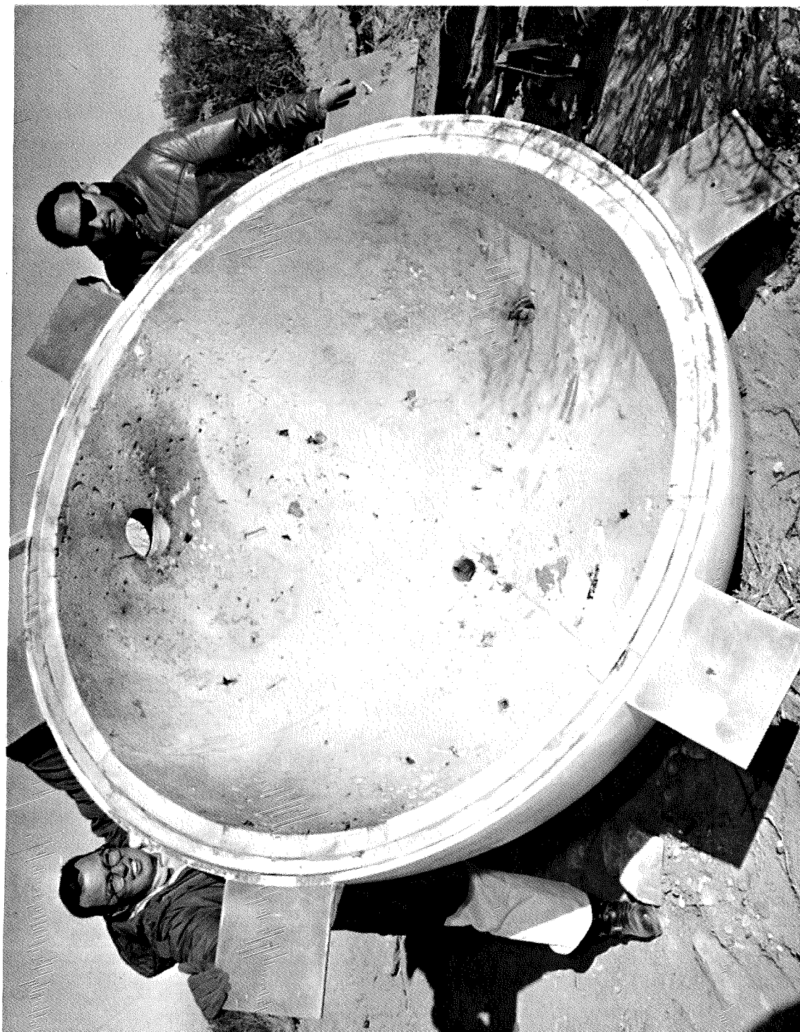
FIGURE 8: Fragmentation on the Dome (One-Eighth Pound Charge)
