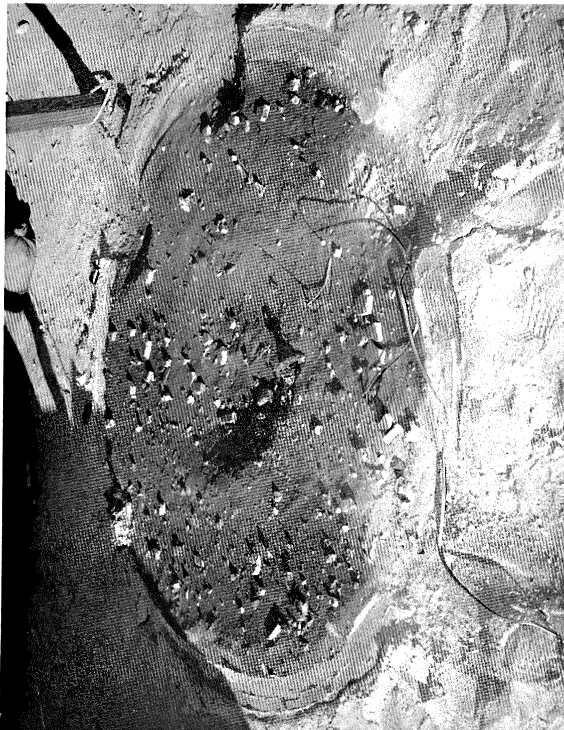
FIGURE 6: Ground After Detonation Under the Dome (One-Eighth Pound Charge)
