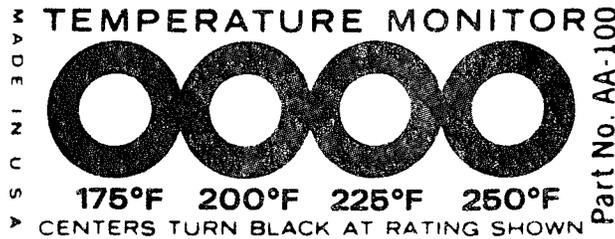
The "Tempilabel" is a temperature monitor consisting of 4 heat-sensitive indicators sealed under transparent, heat-resistant windows. The center of each indicator circle will turn black at the temperature shown. The change to black is irreversible.
