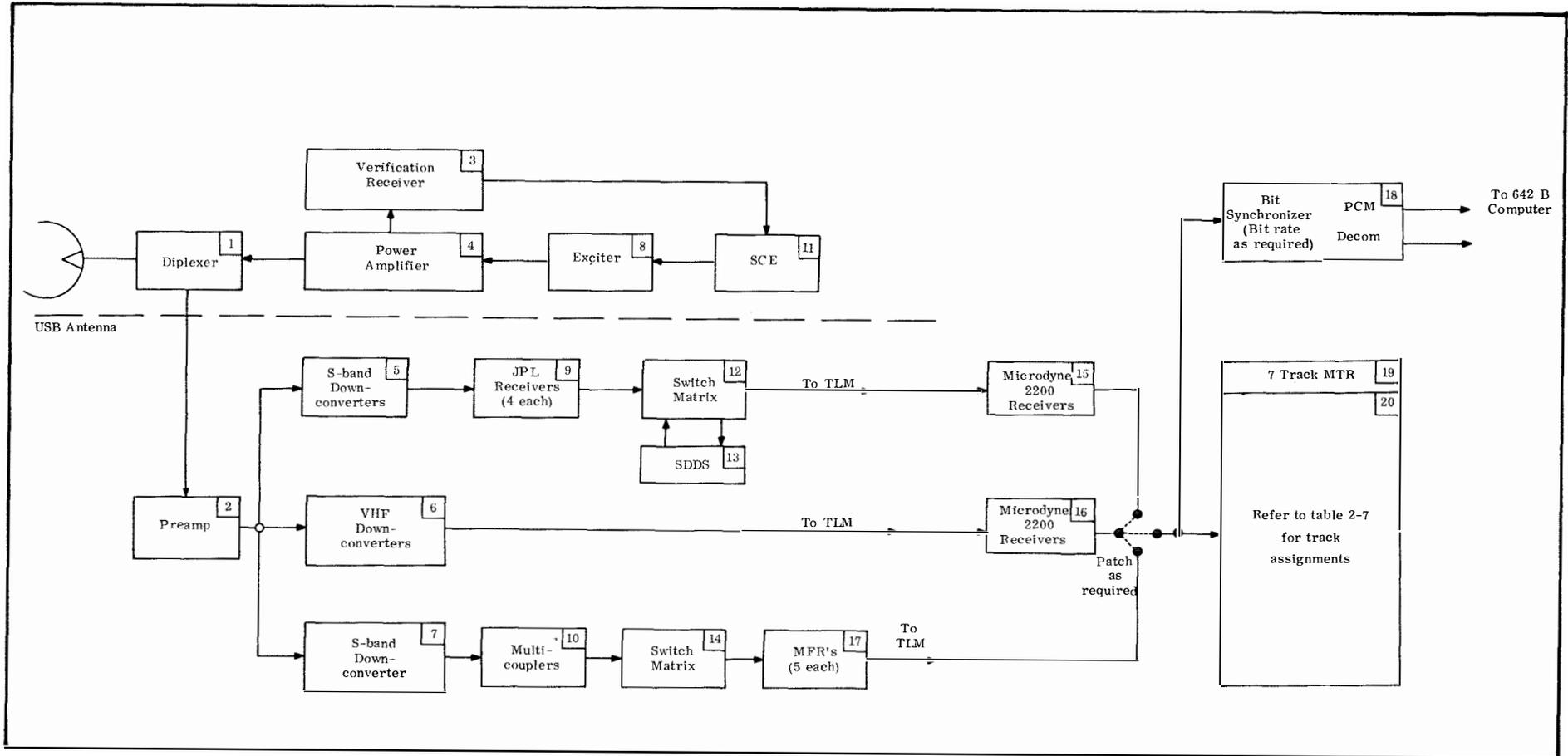
Figure 1-1. 4.3, 9-, and 26-meter ALSEP USB Station Configuration
