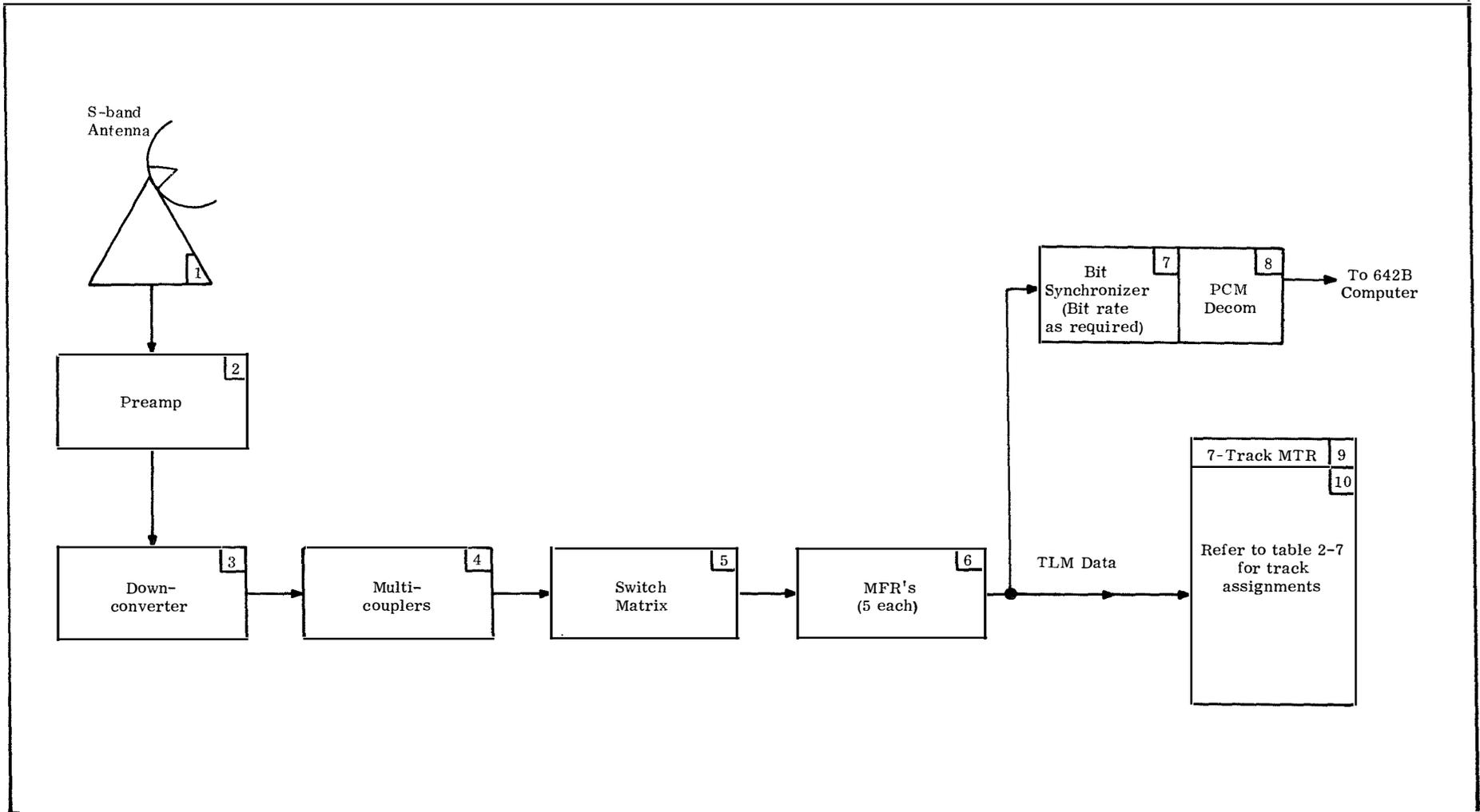
Figure 1-2. 12- and 26-meter ALSEP S-band Station Configurations
