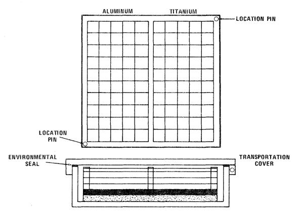
Figure 2. Schematic Plan of FLEA Package
