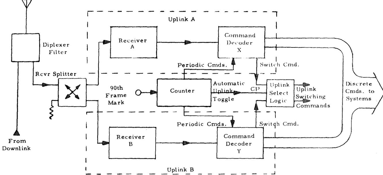
Note: Only Uplink A or Uplink B powered at any one time
