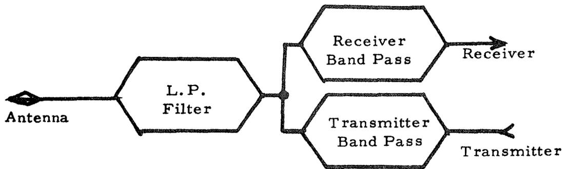
Figure 4-28 Block Diagram of Diplexer Filter
