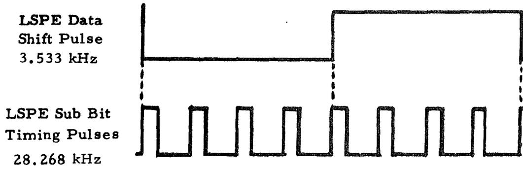
Figure 4-23 LSPE Timing Pulses
