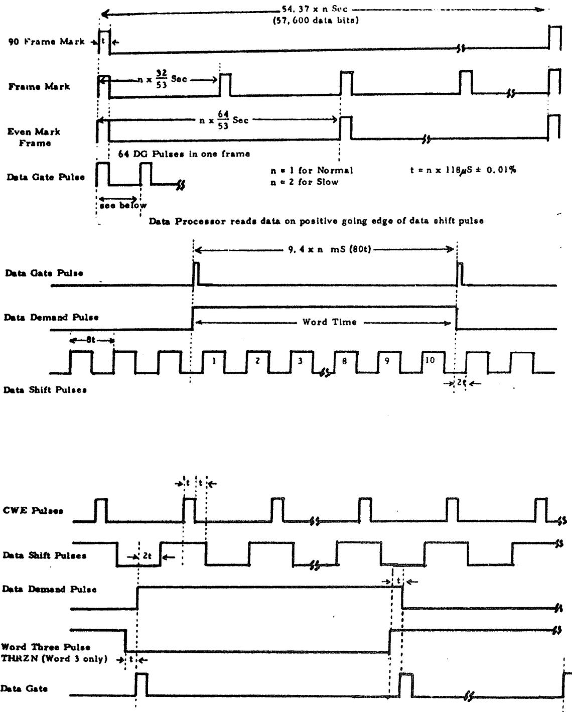
Figure 4-22 DDP Timing Pulses
