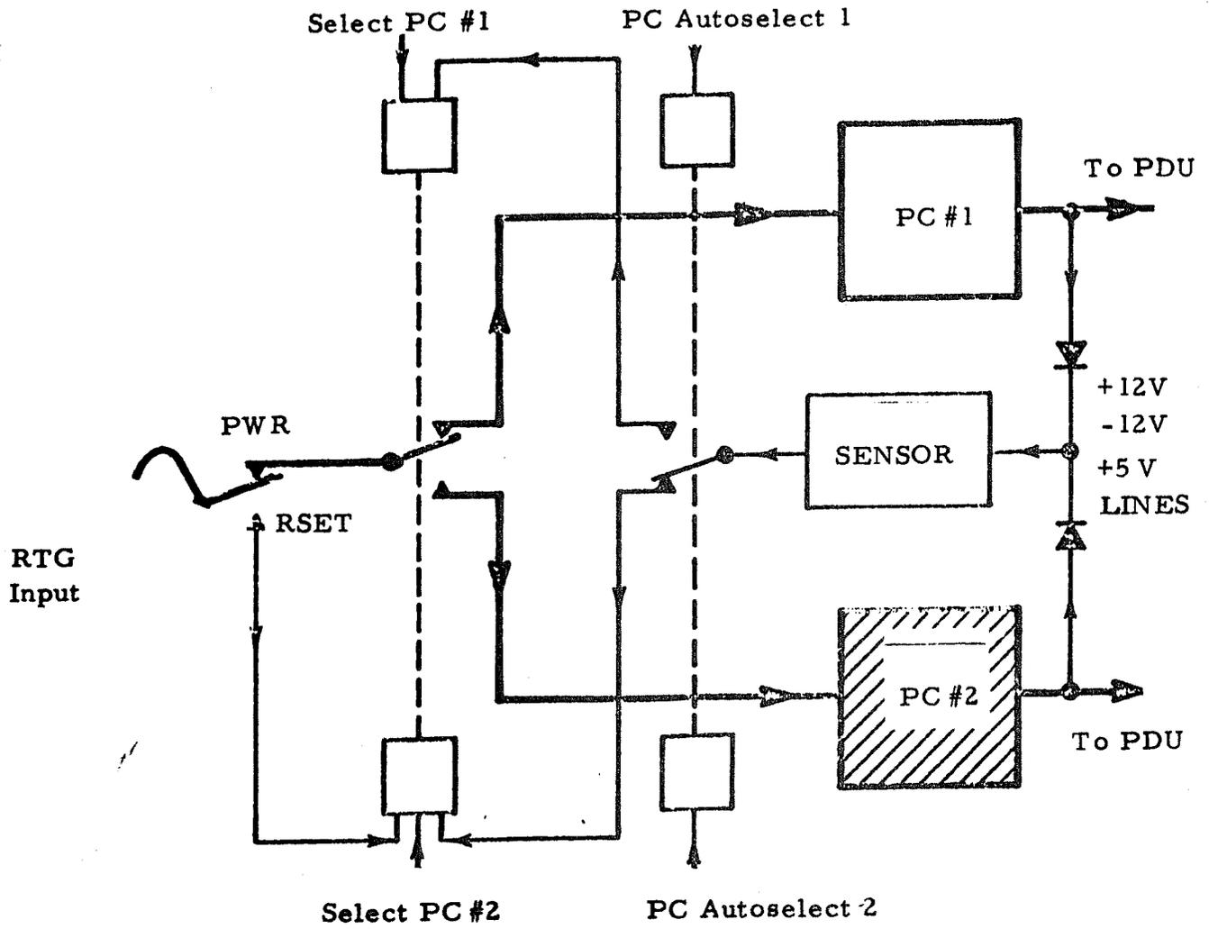
Figure 3-3 PCU Auto Switch Circuitry
