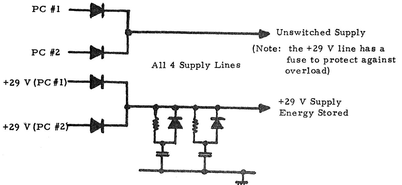
Figure 4-7 Data Subsystem Unswitched Supply Lines
