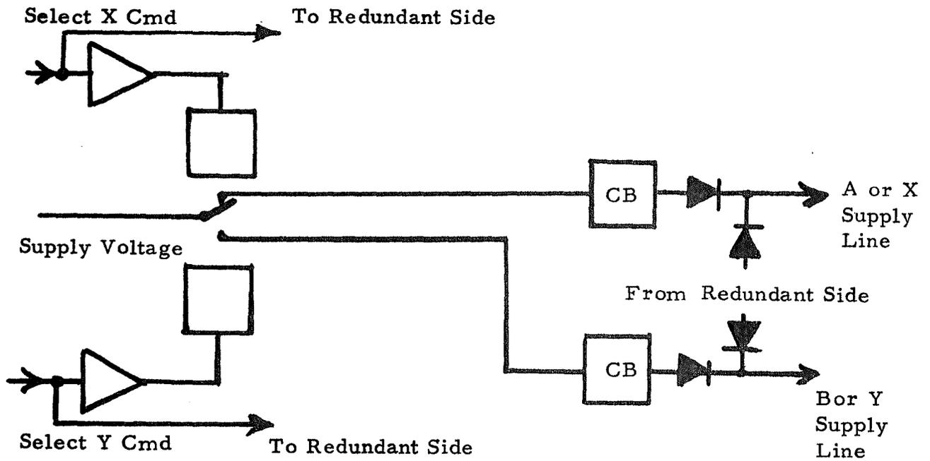
Figure 4-1. Transmitter/DDP Power Control
