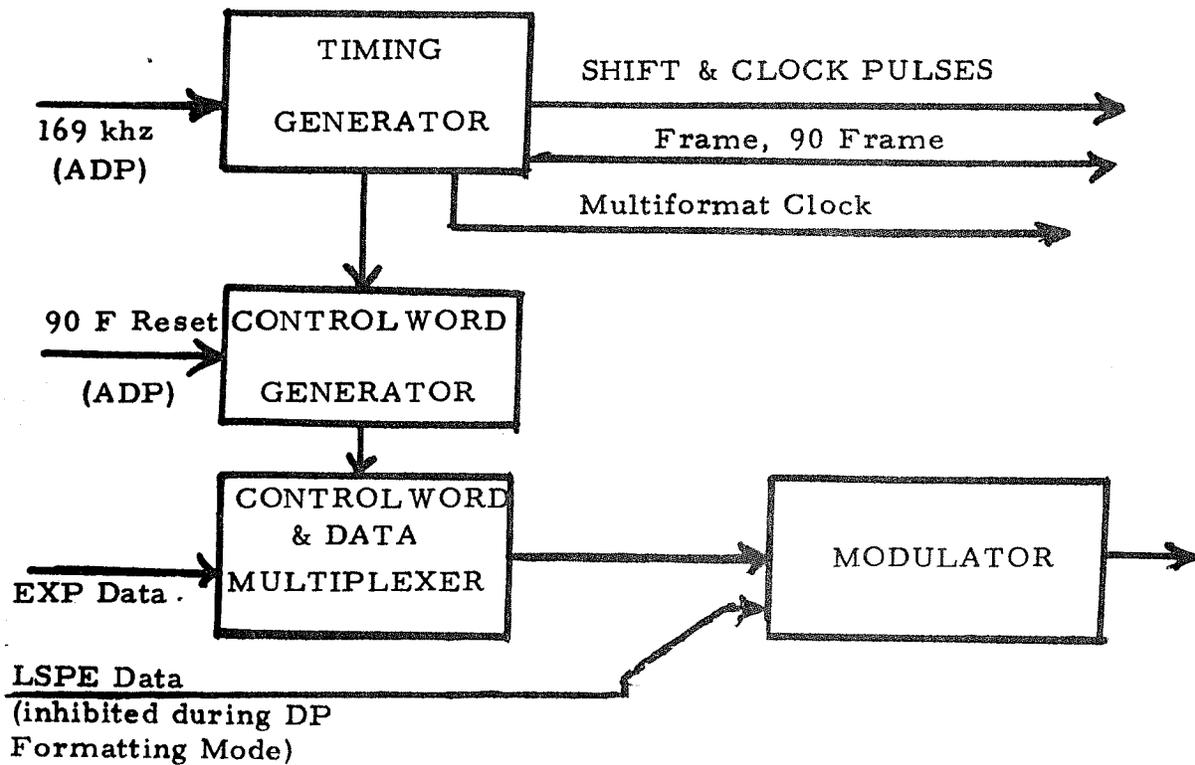
Figure 4-21 Timing and Control Word Generator
