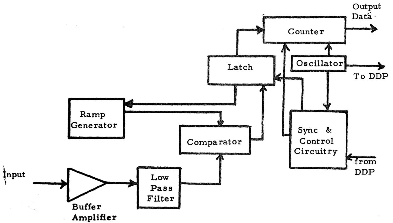
Figure 4-16 ADC Block Diagram
