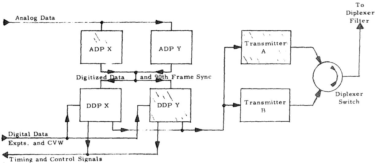
Note: Power to energise any combination of ADP, DDP and Transmitter may be selected by ground command.
