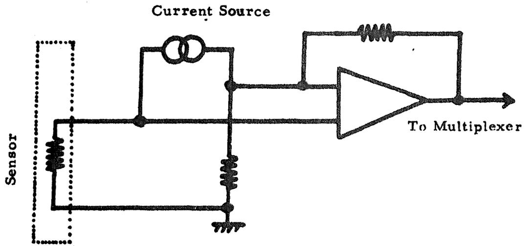
Figure 4-18 RTG Temperature Sensing Circuitry
