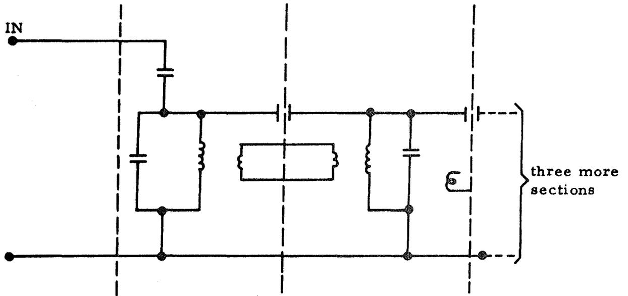
Figure 4-30 Bandpass Filter Equivalent Circuit
