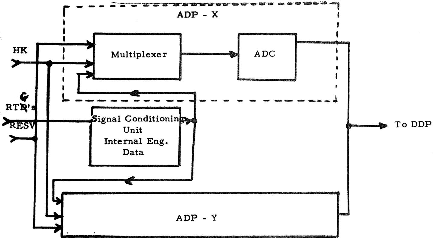
Figure 4-14 Analog Data Processor (ADP)
