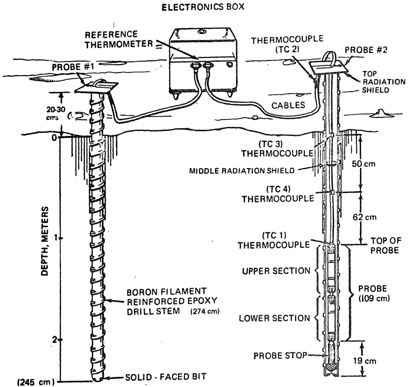
Figure 5-7 Heat Flow Experiment Deployed Configuration
