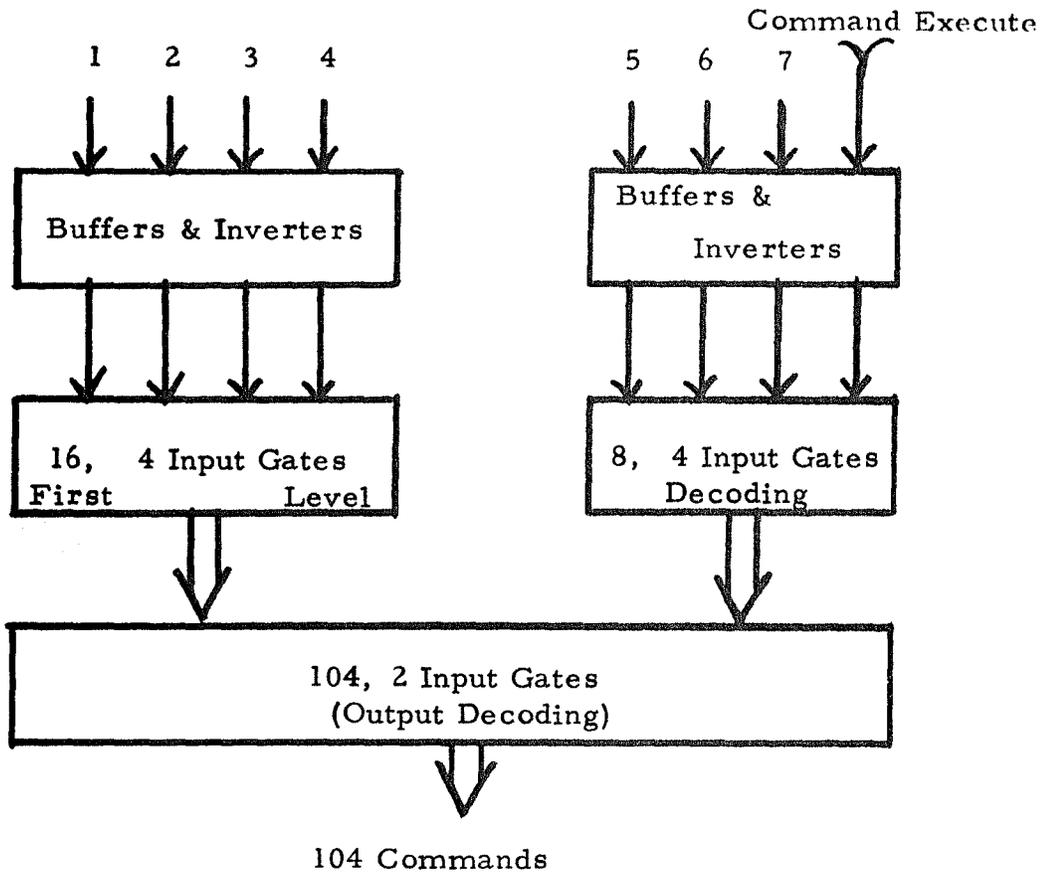
Figure 4-11 Decode Gates
