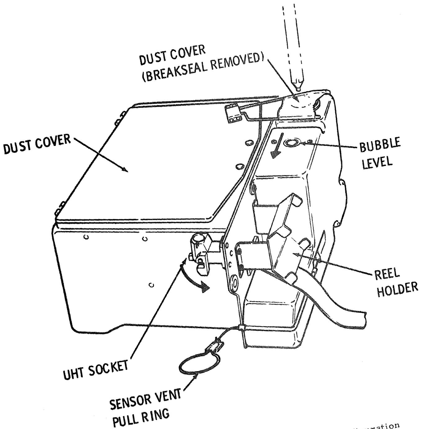
Figure 5-1 Lunar Mass Spectrometer Deployed Configuration
