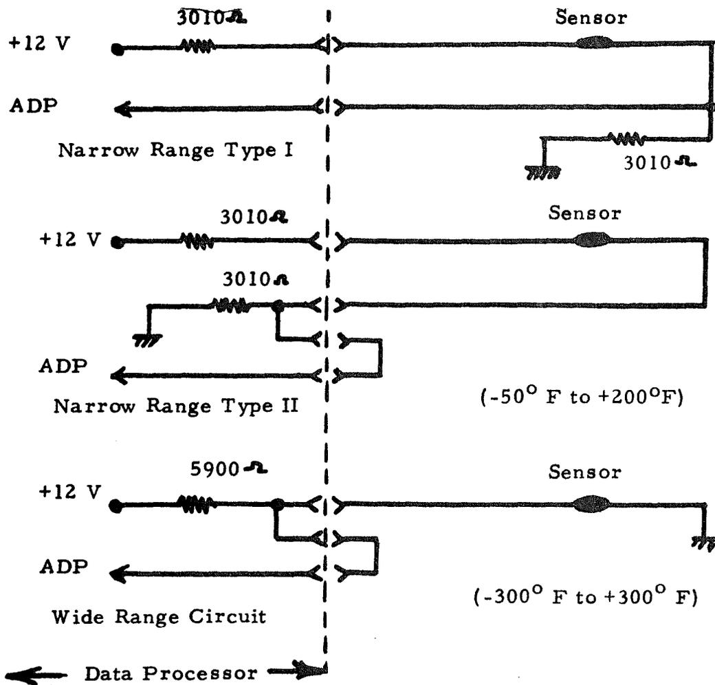
NOTE: The LSP Electronics Internal Temperature Sensor (HK-25) is the only Type II sensor circuit in the ALSEP
