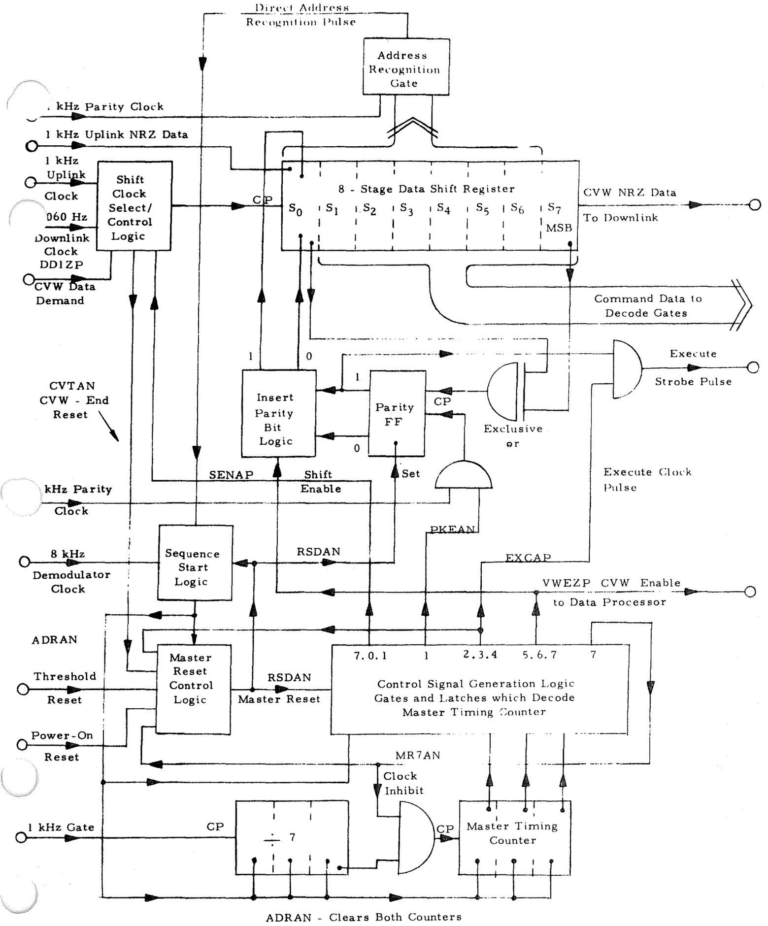
Figure 4-10 Control Logic
