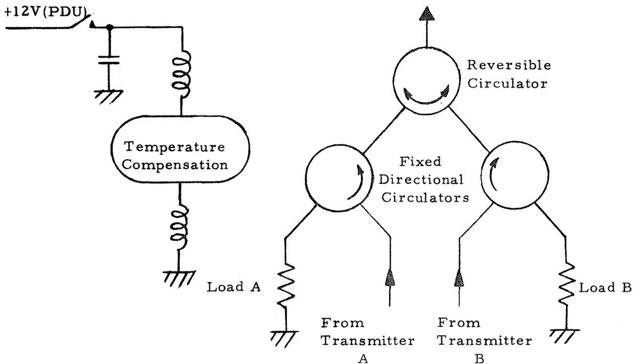
Figure 4-31 Circulator Switch Block Diagram
