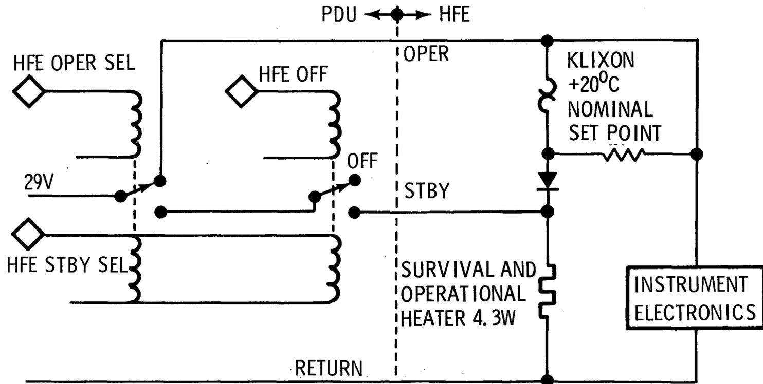
NOTE: ADDITIONAL THERMOSTAT TURNS A PORTION OF INSTRUMENT ELECTRONICS OFF DURING FRAMES 16 THROUGH 89 WHEN TEMP. IS ABOVE 30°C NOMINAL
