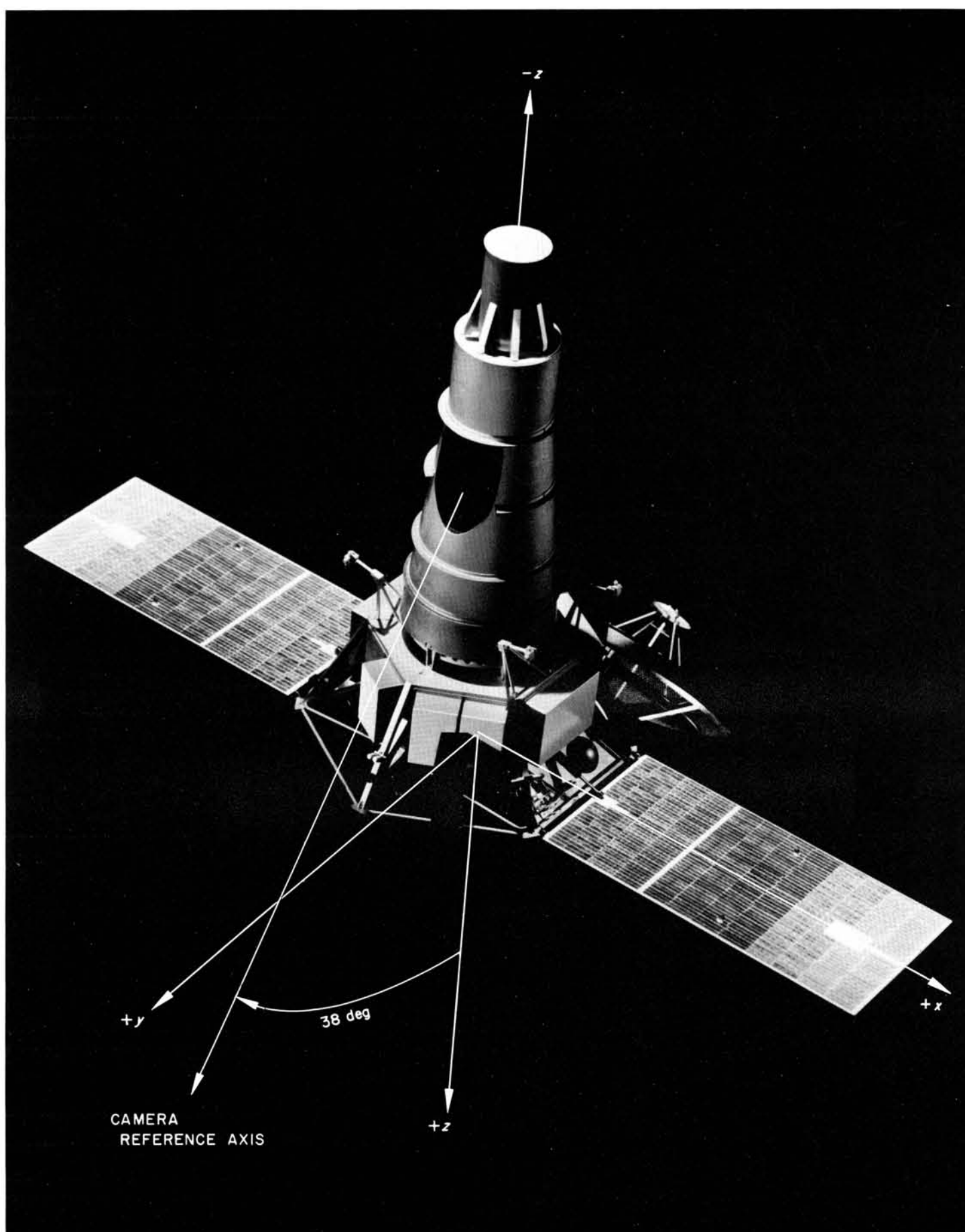
Fig. 2. Spacecraft coordinate system
