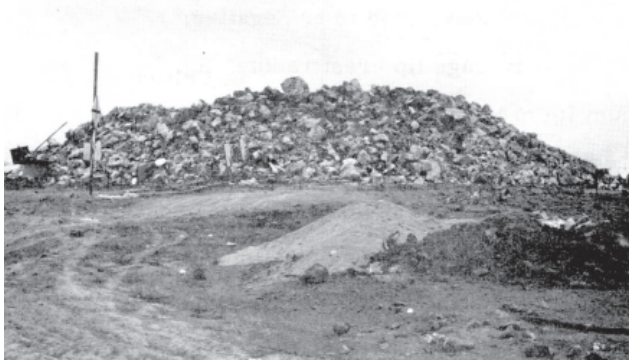
Fig. 6. Side view of the rubble pile produced in a buried nuclear explosion (codename SULKY) in competent basalt. The mound is approximately 46 m in diameter and 8 m high.
