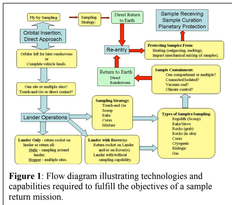
**Figure 1:** Flow diagram illustrating technologies and capabilities required to fulfill the objectives of a sample return mission.
