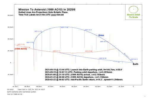
**Figure 2:** An Earth-centered trajectory plot showing a possible 150-day mission profile to NEO 1999  $AO_{10}$  with the CEV on top of an Ares V launch vehicle. Atmospheric re-entry is similar to that of the Apollo missions returning from the Moon. The Moon's orbit is shown for scale.
