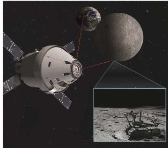
**Figure 2:** Illustration of the NASA Orion vehicle and ESA service module in the Earth-Moon L2 location above the lunar far side, from where crew can tele-operate a sample-collecting rover and maintain communications between surface assets and mission control on Earth.
