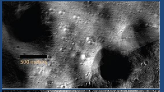
An area (latitude 85.6° north) before and after (upper and lower) control of 7 images, and shown at a resolution of 7.5 m/pixel. Largest shifts are 165 m.
