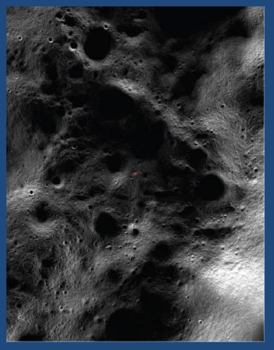
Comparison of LMMP mosaic (left) to current mosaic (right), at 11 m/pixel, covering 11.4 x 5.7 km. The red dot is the north pole. The central region here was shown previously. The oddly sharp edges to features in the left image are due to automatic removal of low SNR portions of images in the averaged LMMP mosaic. The darker areas in the right image are due to the lack of such editing and the averaging of many dark images in the current mosaic. Which is best?
