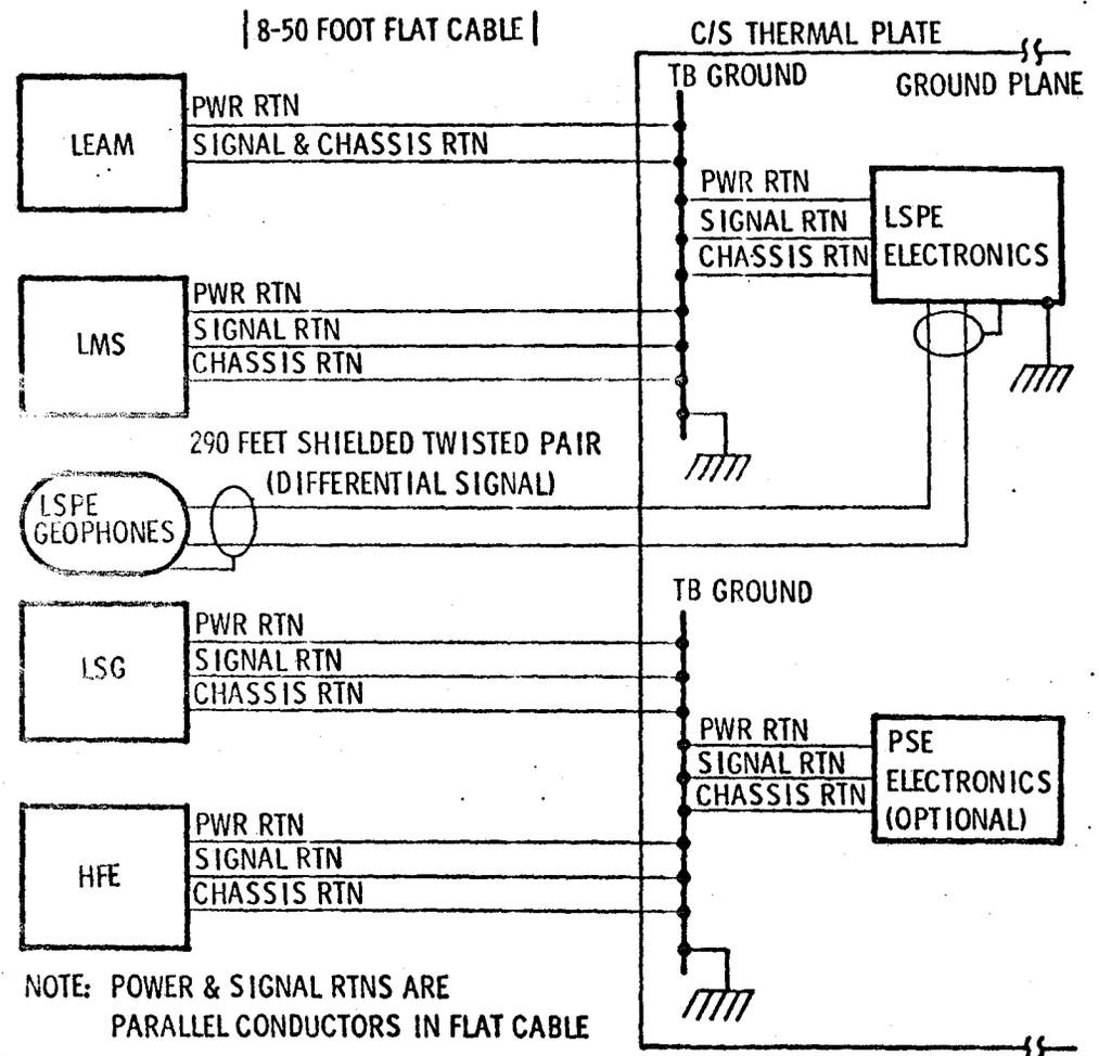
NOTE: POWER & SIGNAL RTNS ARE PARALLEL CONDUCTORS IN FLAT CABLE
