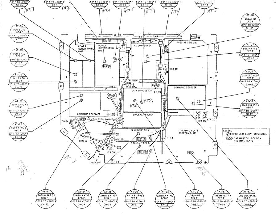
Figure 1 - ALSEP Central Station Thermal Plate Thermistor Locations
