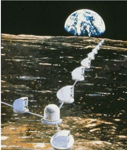
Figure 4. Lunar optical interferometer. The individual telescopes send light to the central beam combination dome, where the interferogram would be constructed. Individual telescopes could be separated by 100 to 1000 meters.
