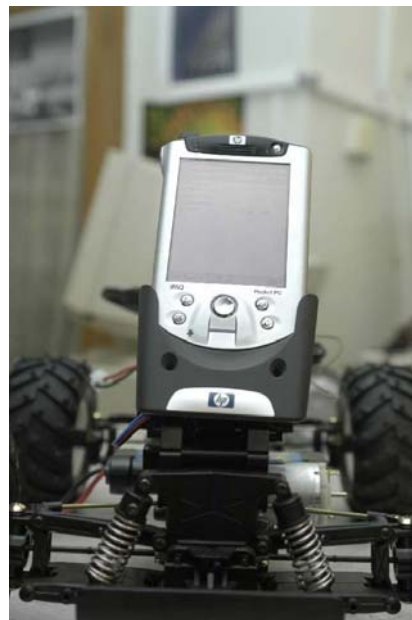
Fig. 2. Husar-2a for college students. Second level. The DPA computer on the front of the rover.
