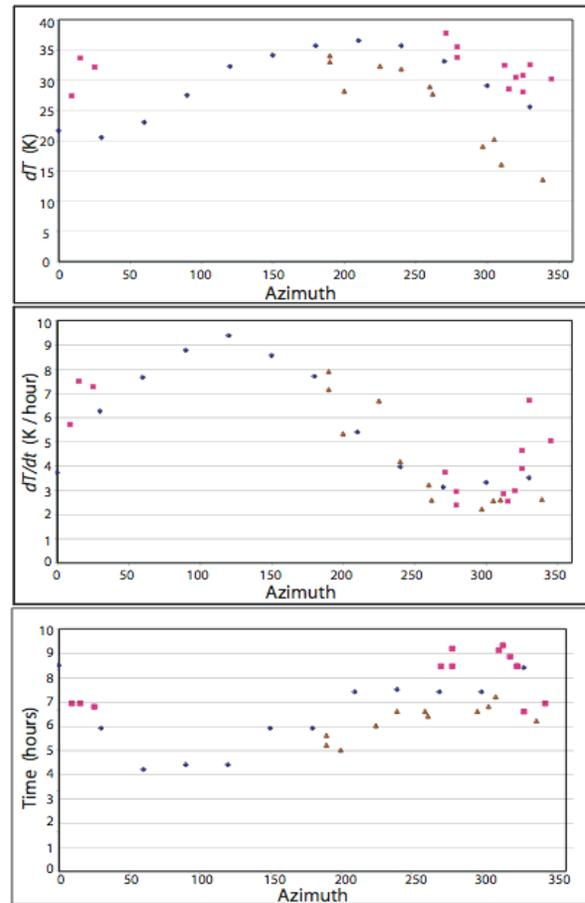
Figure 3: Measured parameters extracted from diurnal thermal curves from multiple facets on all three dune targets (Eureka dunes in blue diamonds, Dumont Dunes in orange triangles, and the model dune in pink squares): a) Difference between maximum and minimum temperature ( $\Delta T$ ) as a function of slope azimuth; b) Morning heating rate ( $dT/dt$ ) between 7:30 am and 9:30 local time; c) Time between minimum and maximum temperature ( $\Delta t$ ) in the morning.
