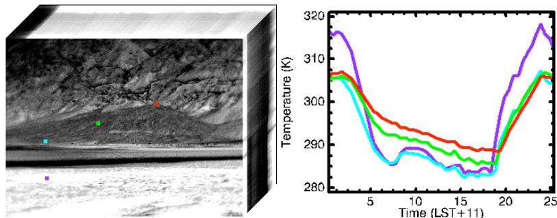
Figure 5: A thermal image from a hypertemporal image cube of a debris-flow dominated alluvial fan (left), with associated diurnal temperature curves for selected locations (right). Colored dots on left indicate the locations of the correspondingly-colored diurnal curves on the right.
