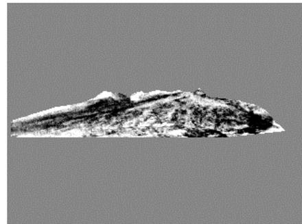
Figure 6: A principle component (PC) band from the hypertemporal cube shown in Figure 5. Pixels not on the fan were masked for the PC transformation.
