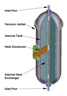
tank with removable domes. An internal, finned heat exchanger evenly added and removed heat from the sorbant bed. A centrally located heat conductor provided the transfer point for external cooling. Flow through the bed was enhanced with an central flow distribution bar and an outer screen plenum to minimize pressure drop.
