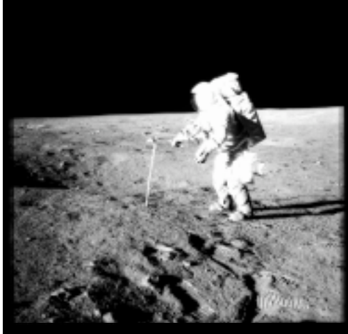
Photo Credit: Pete Conrad for NASA. Figure 1. Apollo 12 astronaut Alan Bean obtaining a lunar core sample. Apollo drill cores were very useful in providing information about impact gardening and surface exposure effects on the Moon.
