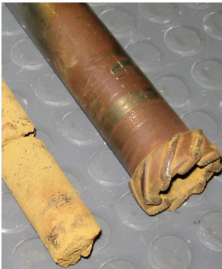
Photo Credit: Kiel Davis for Honeybee Robotics. Figure 2. Mars Deep Drill Bit & Core Sample. This system is being developed for automated drilling and coring in frozen, planetary environments by Honeybee Robotics.
