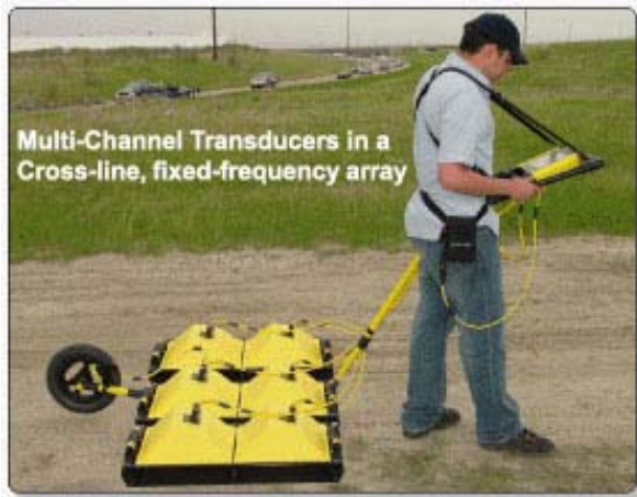
Figure 3. Multichannel bistatic configuration [2]
