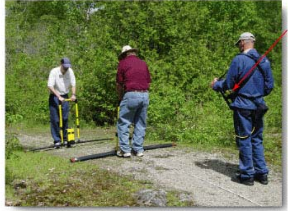
Figure 4. CMP velocity sounding [2]
