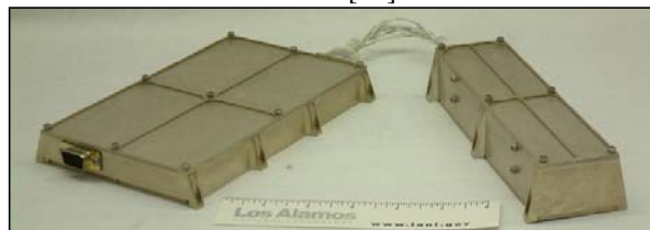
Figure 1. Miniature neutron spectrometer; neutron sensors are in the sensor module (right). Associated electronics are in the data module (left). The mass of both modules combined is 484 g.
