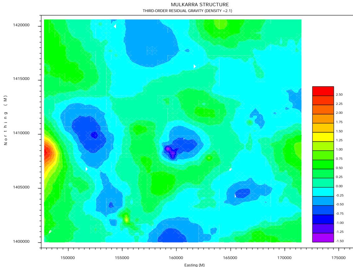
**Figure 1.** Color coded contour map of the third order residual gravity. Reduction density was  $2.1 \text{ g cm}^{-3}$ . A  $50 \times 50$  grid was calculated and contoured. Contour interval is  $0.25 \text{ mGal}$ .
