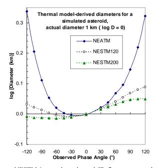
NESTM is tested on thermal IR fluxes generated from simulated asteroid surfaces with different  $\Gamma$ . NEATM and NESTM diameters are compared with radar diameters, and it has been found that NESTM may reduce a systematic bias in overestimating diameters. From these tests, it is suggested that a version of the NESTM which assumes  $\Gamma = 120 \text{ J m}^{-2} \text{ s}^{-1/2} \text{ K}^{-1}$  is adopted as a default model when the solar phase angle is greater than  $45^{\circ}$ .
