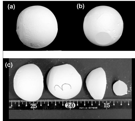
Fig. 1 Porous gypsum targets. (a) Original, (b) compacted, and (b) fragmented spheres of 50 mm in diameter. The impact velocities were (b) 10.2 m/s and (c) 22 m/s.
