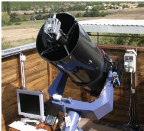
Fig 2 : the telescope MOSS with the camera at the prime focus.
