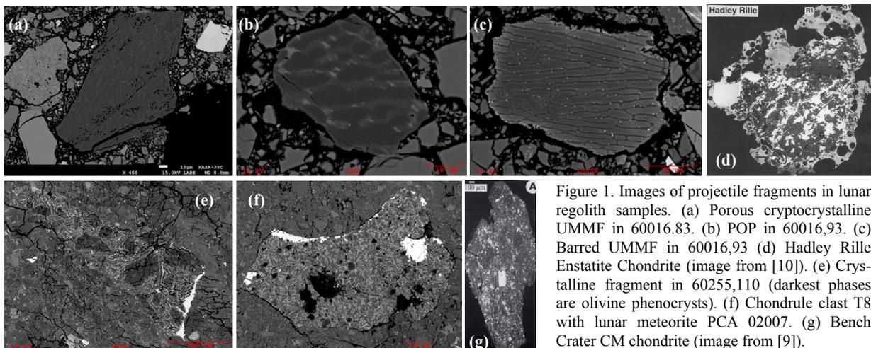
Figure 1. Images of projectile fragments in lunar regolith samples. (a) Porous cryptocrystalline UMMF in 60016.83. (b) POP in 60016.93. (c) Barred UMMF in 60016.93 (d) Hadley Rille Enstatite Chondrite (image from [10]). (e) Crystalline fragment in 60255,110 (darkest phases are olivine phenocrysts). (f) Chondrule clast T8 with lunar meteorite PCA 02007. (g) Bench Crater CM chondrite (image from [9]).
