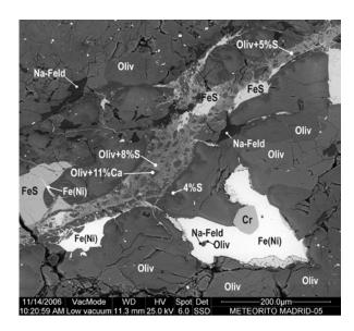
ESEM-BackScattering Image showing a schock vein composed by a mixture of Olivine, Troilite and infilled iron in very thin veins sized from 1 to 3 microns.
