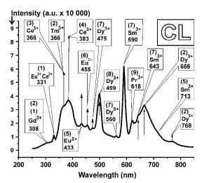
This merrilite (CaPO<sub>4</sub>) from Madrid L6 Chrondrite emits cathodoluminescence peaks attributed to Ce<sup>3+</sup> (360-380 nm peak), Dy<sup>3+</sup> (499 nm peak and 666nm peak), Sm (590 nm peak) and Tm<sup>3+</sup> (366 nm peak).
