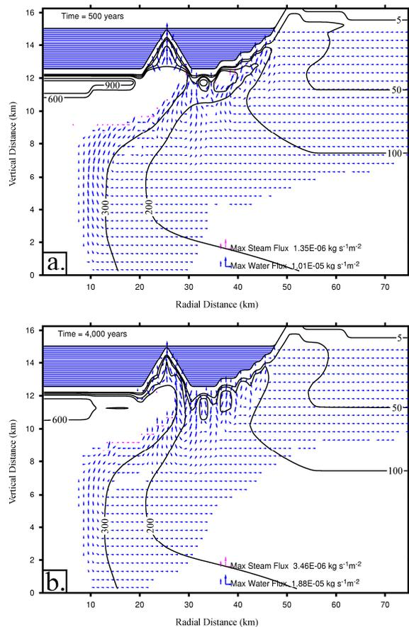
**Figure 1.** Results of a numerical simulation of the hydrothermal system at a 100-km impact crater on early Mars. Surface permeability is  $10^{-2}$  darcies. Black lines are isotherms, labeled in degrees Celsius, and blue and red arrows represent water and steam flux vectors, respectively. The length of the arrows scales logarithmically with the flux magnitude, and the maximum value of the flux changes with each plot.
