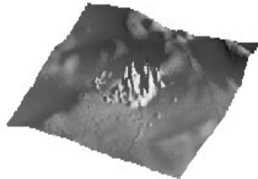
**Fig. 1.** Total magnetic-field intensity over Steen River impact structure. Compare short wavelength crater anomalies to broader regional anomalies.
