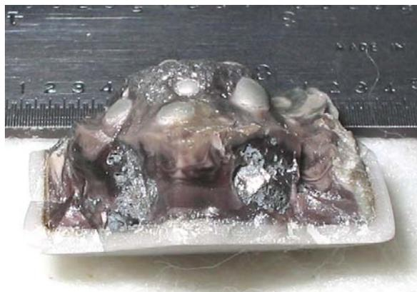
**Figure 2:** JSC-1 carbothermal reduction residue.
