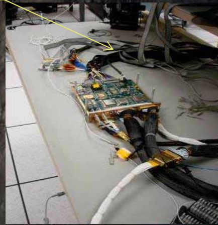
Successful Interface testing between Coarse Sun Sensor (CSS) and Multipurpose Access Card (MAC).
