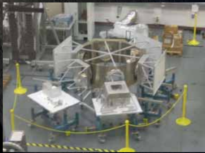
LCROSS harness fabrication in process using structure mock-up.
