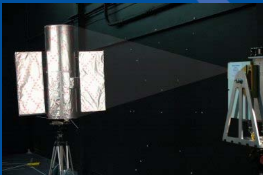
TriDAR: Lidar combined with triangulation
