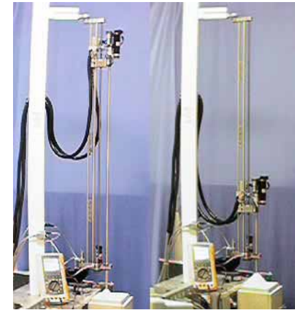
SATM Prototype Drilling into Chalk Sample
