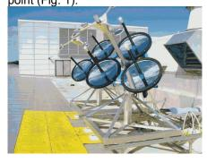
Collected PAR is transmitted through 10-m-long fiber-optic bundles that deliver 40-50% of the original solar radiation to overhead emitters in a growth chamber.
