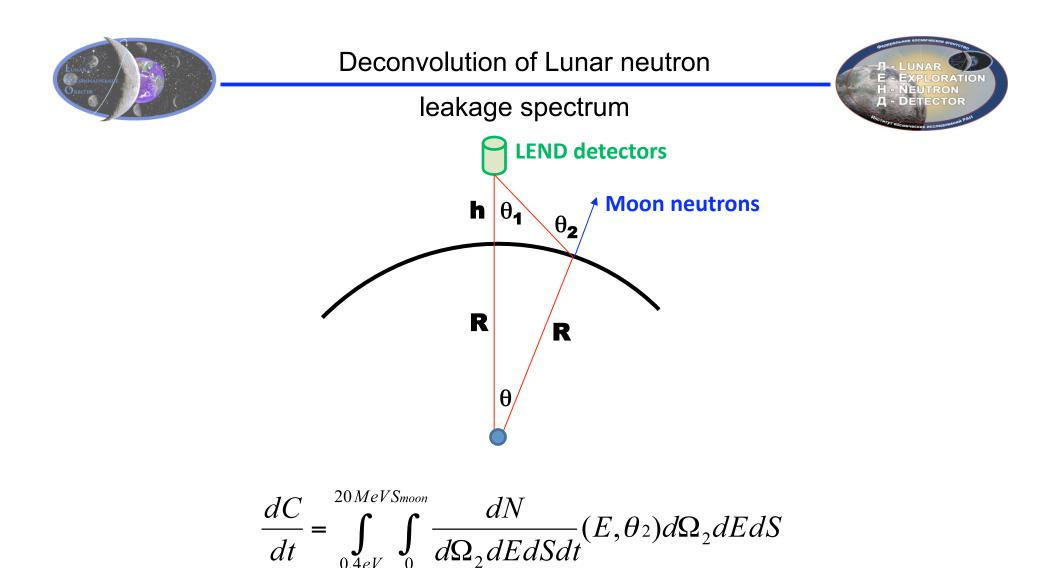
Where dC/dt – counting rate (counts per second) detected by LEND neutron sensors
