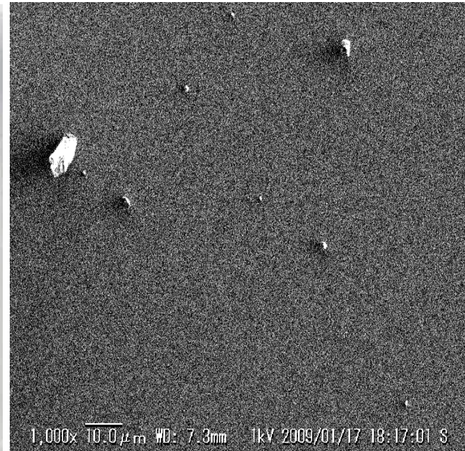
Residual Dust on Conveyer after Cleaning Operation
