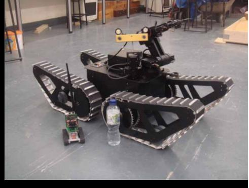
SELENE did not manage to freedom robot arm locomotion drives turned out to be undersized
