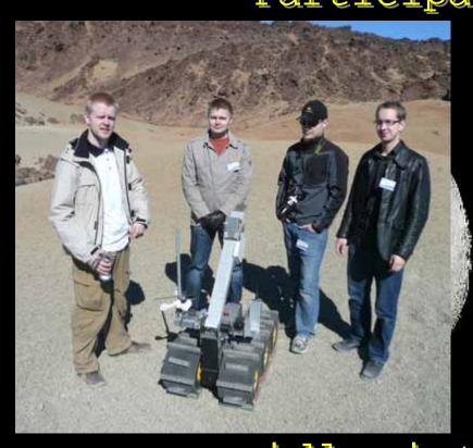
The Oulu robot went very rapidly into the crater. Unfortunately as it did not have a communication relay on the rim it lost communication with the "ground station" while climbing
