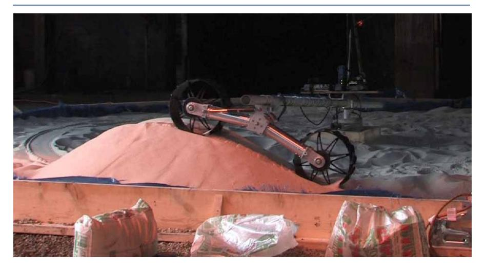
Wheel and drive train are being run tens of kilometers in simulated lunar soil using counterweighted boom to mimic one-sixth gravity of the Moon
