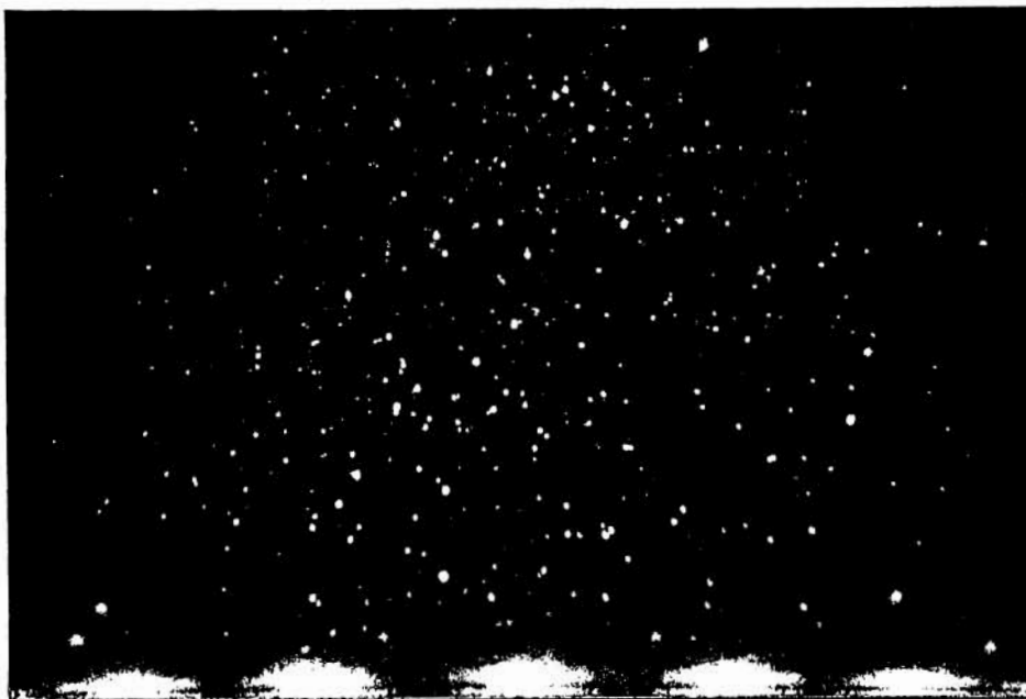
Fig. 2 \sim 300 m/sec particles embedded in solid xenon film ( \sim 0.3 mm thick) at -188 C. Some of the particles are not in focus because they end up at various depths in the film. The full picture represents an actual area of \sim 10 mm 2 .
