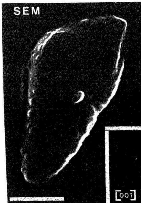
FIGURE 2: SEM and TEM images and SAED pattern [inset; d(010) = 10.29\text{\AA} ; arrowed] of a Solar Max olivine particle. Bumps (SEM image) and inclusions (TEM image; arrowed) are an Fe-Ni phase. (NOTE: central bright spot in SEM image results from electron beam contamination).
