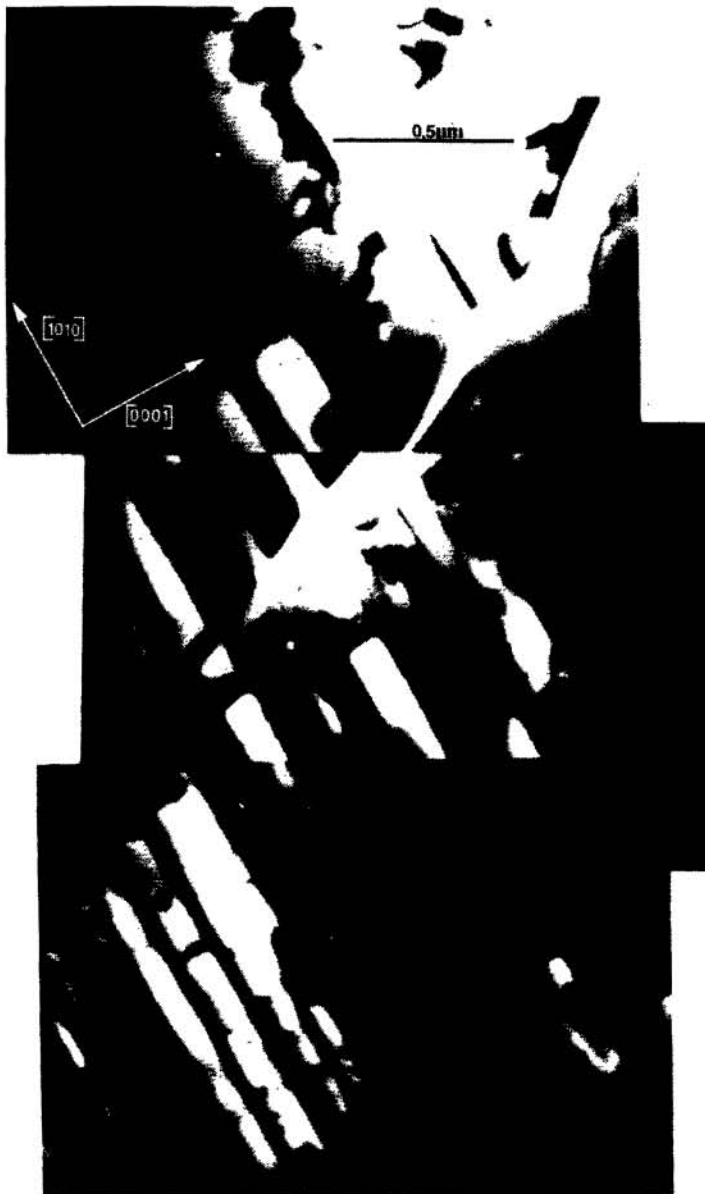
Figure 1: Electron micrograph of shock lamellae formed at 12 GPa. Lamellae are dominantly basal; some are wedge-shaped. They are connected to a glassy vein (bright area, upper right), and generally thin away from it, in places reconnecting.
