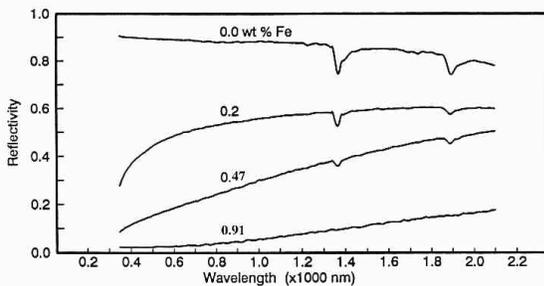
**Figure 2.** Results of Allen's lunar soil analog for various wt% Fe implaced in silica gel particles [12].
