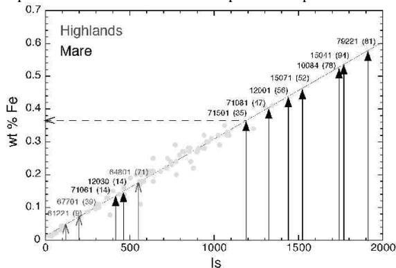
**Figure 3.** Relation between  $I_s$  and Wt% Fe derived from lunar soils [morris ref]. The arrows show the <10 $\mu$ m  $I_s$  values which can then be extrapolated in order to obtain estimates for the weight percent of nanophase Fe present in each sample. Solid arrows indicate mare samples, open arrows represent highlands. The soils are labeled with their sample number followed by their bulk soil  $I_s/FeO$  value.
