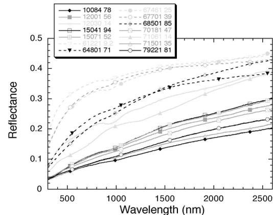
**Figure 1.** Bi-directional reflectance spectra of the <10 $\mu$ m samples used in this study. Solid lines are mare, dotted are highlands. Light gray represent immature soils, dark gray = submature, and black = mature. The bulk soil I<sub>v</sub>/FeO values are given in the legend.
