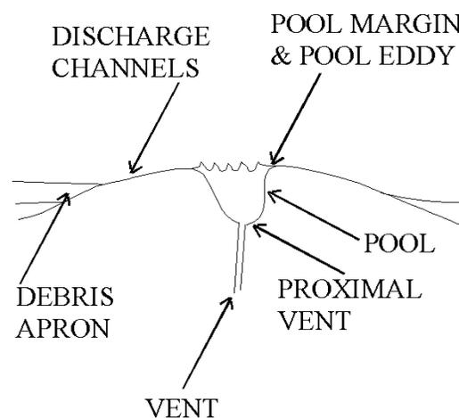
Figure 1: Generalized schematic cross-section through a subaerial hotspot deposit showing major facies.
