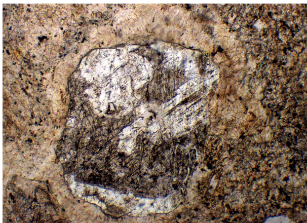
Fig.1. Optical micrograph of shocked quartz altered by zeolite mineral at Miura (Kagawa-Takamatsu) crater in Japan. 1.5mm horizontal size of the micrograph [5, 8].
