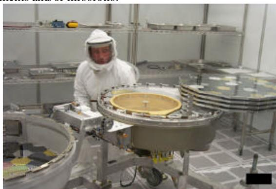
**Figure 4:** R. Paynter/JPL checks the precision-cleaned and fully reassembled Genesis science canister.
