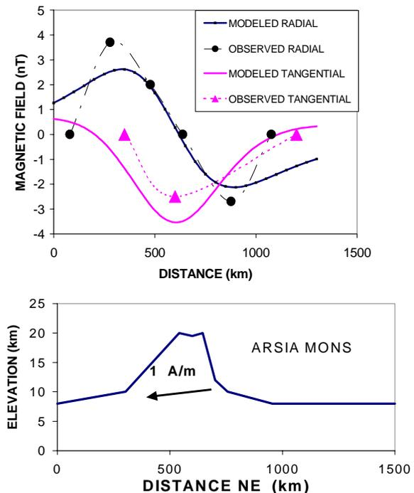
Figure 4. Modeled and observed magnetic field profiles 400 km above Arsia Mons along the profile line indicated in Fig.2. The observed radial values are directly from the residual map (Fig.2). The observed tangential values of the residual anomaly were estimated by inspection of Fig. 3. The topography and magnetization vector used in the model is shown in the lower panel.
