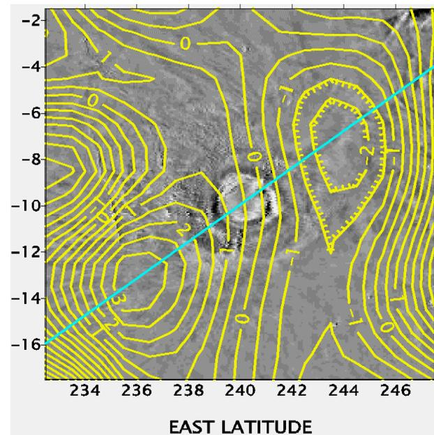
Figure 2. Radial magnetic residual anomaly map superimposed on Arsia Mons. The contour interval is 0.5 nT. Closed negative contours are hatched. The line of inferred magnetization is also shown.
