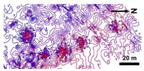
Figure 3. Intensity of total magnetic field of a section of the crater field. Mapped craters are indicated by dashed circles.
